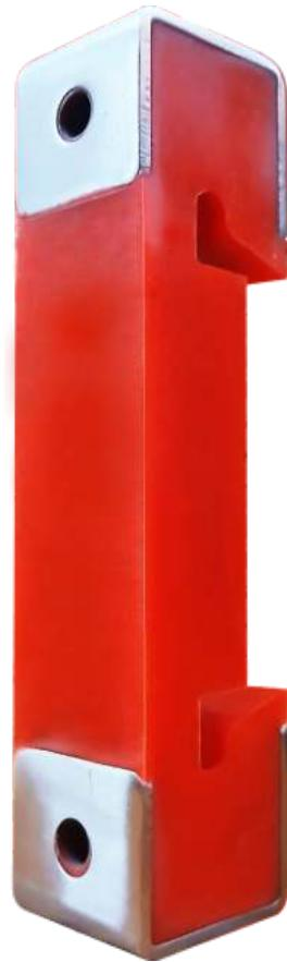
EasyGrip Sound Furring Clip resiliently secures common drywall furring channel. Offering significantly higher STC values than drywall attached to resilient channel, EasyGrip ensures that installers will not inadvertently screw through the "resilient" leg of the channel into the joist or stud.
